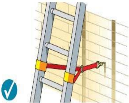
Tying near the base
