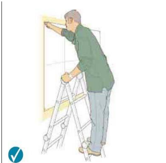
Correct – two clear rungs. Don't work any higher up this type of stepladder.
